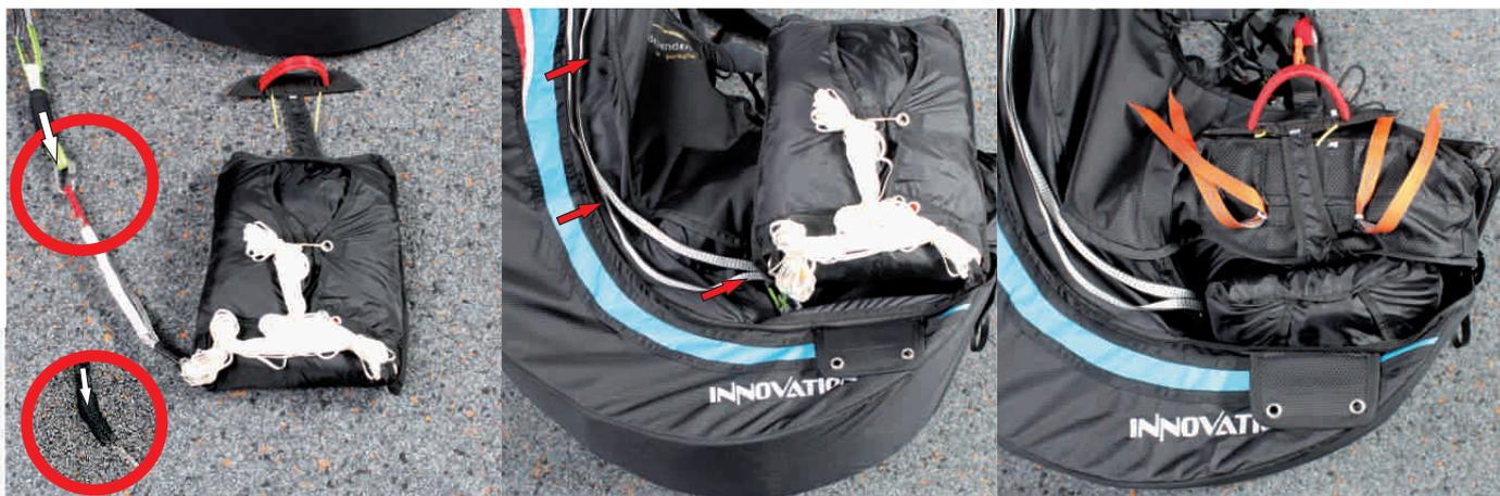
1. Connect the rescue bridle with the harness bridle by looping the bridles or with a quick link (strength > 2400 daN) and fix the connection to prevent slipping (for example by a neopren sleeve).
