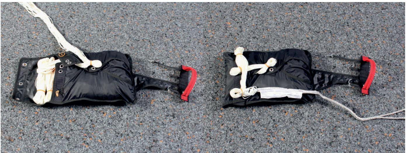
4. Close deployment bag with the lines. First the right flap with the upper and lower flap. Depending of the rescue system size the inner or outer grommets can be used to adjust the container volume.
