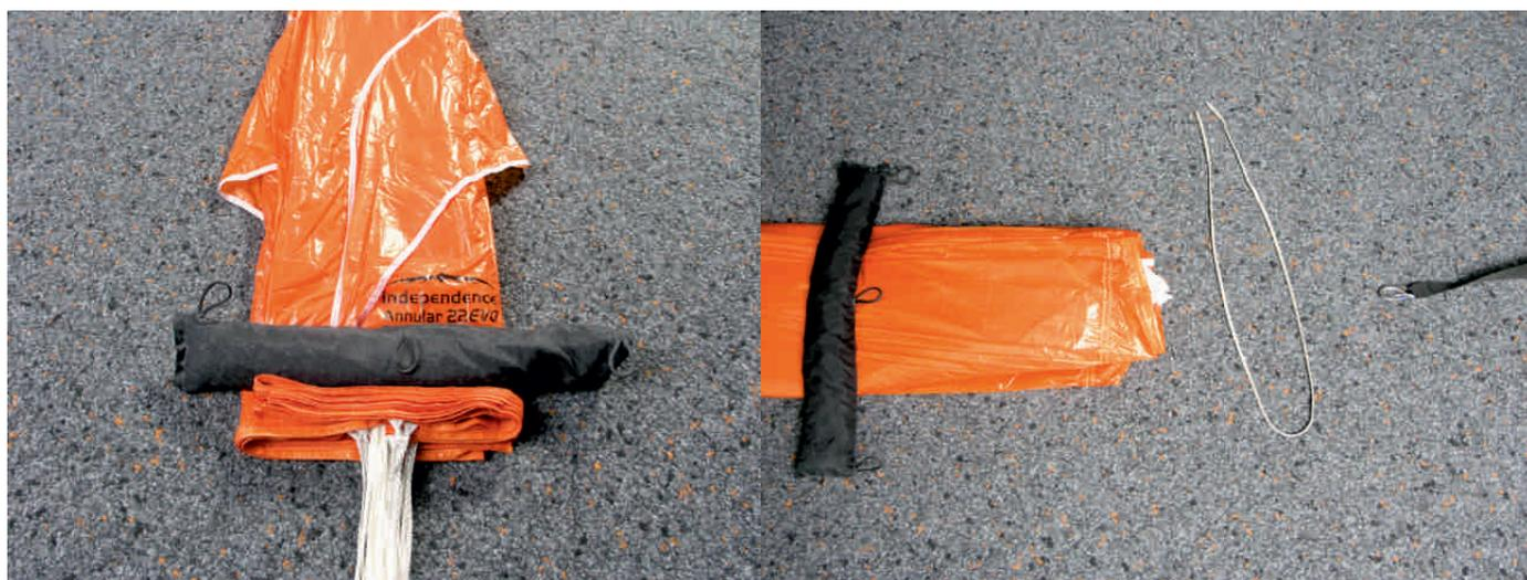
1. Fold the parachute like a "S" on the width of the container, pull out the Ram-Air-pockets a little bit to the side (if the parachute is equipped with Ram-Air-pockets).
